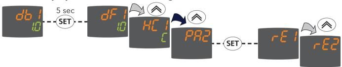
Press the set key next to the desired folder ("rE2" in the example), the first parameter contained in the folder will be displayed. Select the desired parameter using the and keys. Change the value (shown on the second line) using the and keys, then press the set or fire keys to store the new value.
