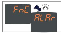
After pressing the fine key, you can scroll through the two folders in the menu (FnC and ALAr) using the and keys.
