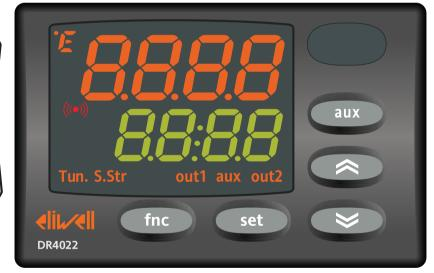
**NOTE**: If "Upper" **PV** DISPLAY is FLASHING the value of "Lower" **SV** DISPLAY is editable.
