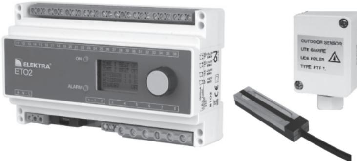
ELEKTRA ETOR2 controller – as standard, equipped with one air temperature sensor and moisture sensor. Additional moisture sensor can be connected to this controller, which will enable protection of two independent roof areas.
