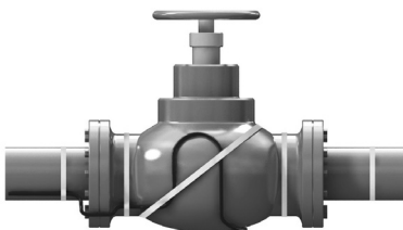
Installation of a self-regulating heating cable on valves
