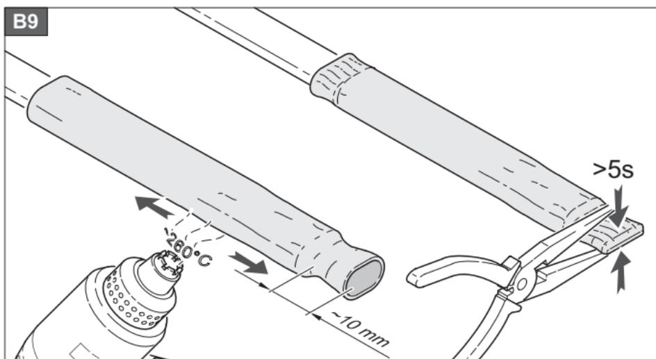
Shrink the tube using the hot air gun
