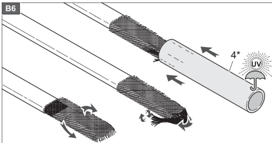
Unroll and twist the protective screen over the heat-shrink tube recreating insulation.
