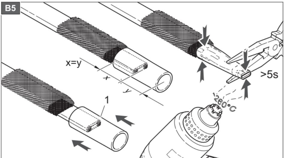
Pull the heat shrink tube 1 (fig. Z1) up to mid-length.
