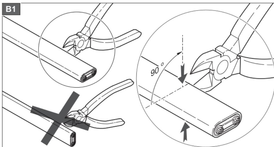
Cut the end of the heating cable straight, or cut off the original protective cap (the protective cap does not constitute the correct reconstruction of the cable's insulation).
