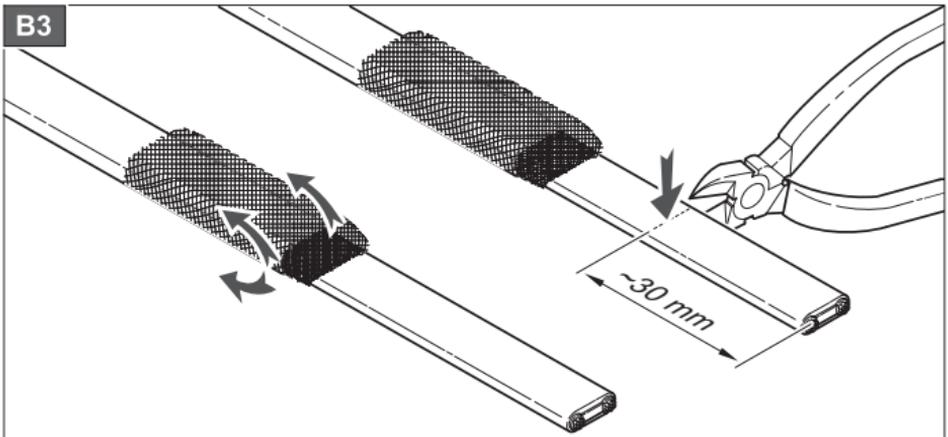
Curl away the protective screen onto the cable's sheath. Cut 30 mm of the cable's end (including the electrical insulation, heating element and conductor wires).
