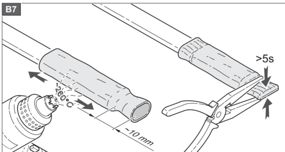
Shrink the tube using the hot air gun (at the temperature  $260^{\circ}\text{C}$ ).
