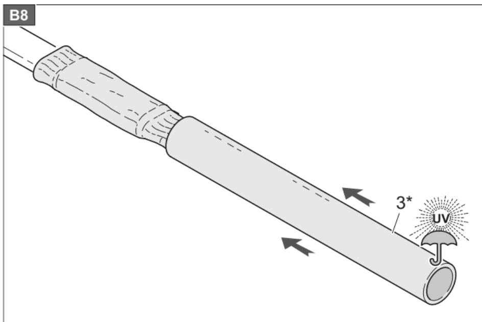
Pull the heat shrink tube 3 (fig. Z1)
